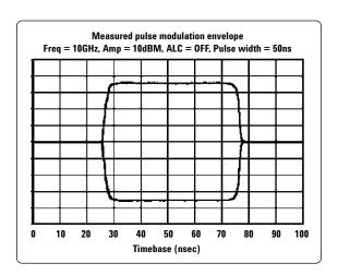
With ALC off, specs apply after the execution of power search. Specs apply with Atten Hold off (default mode), or ALC level between 0 and +10 dBm.
